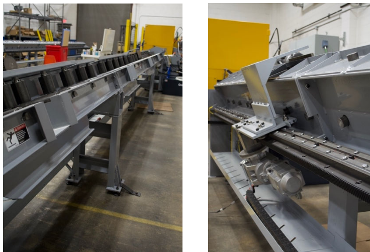
Figure 7: Infeed Conveyor and Pusher/Gripper Assembly
